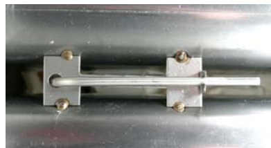
Typical high-limit/sensor probe locations and mounting hardware.
